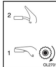
Squeeze the Traction Drive Clutch Lever against the Handlebar (1) to engage wheel drive for propelling unit. Forward speed will vary according to snow depth and moisture content. Release lever (2) to stop movement.
