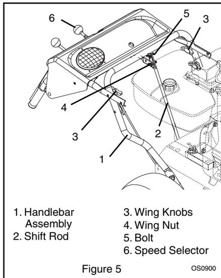
1. Remove lower wing knobs on handlebar assembly (Figure 5).
