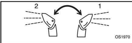
Press the chute rotation switch right (1) to rotate chute clockwise. Press the chute rotation switch left (2) to rotate chute counterclockwise.
