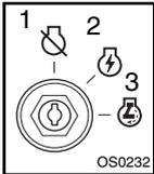
The ignition switch is operated by a removable key. It has three positions:
