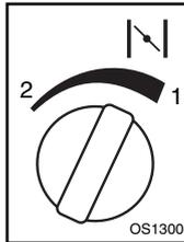
1. Choke Closed position: chokes off air to engine for easier start.
