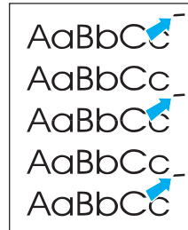
Vertical Repetitive Defects
