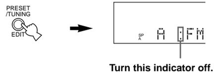
**4** Press PRESET/TUNING  $\triangleleft/\triangleright$  to tune in to the desired station manually.
