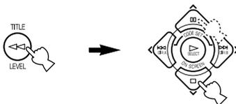
**3** Press  $\langle / \rangle$  to adjust the speaker output level.
