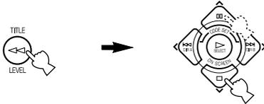
**5 Press </> repeatedly to adjust the output level of the effect speakers so that the output level coming from each speaker is the same.**
