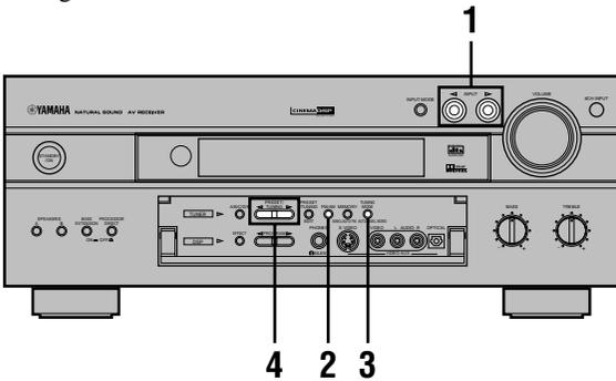
**1** Press INPUT  $\triangleleft/\triangleright$  to select TUNER as the input source.
