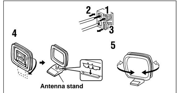
**1** Press and hold the tab to unlock the terminal hole.
