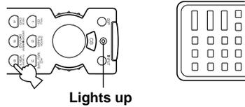
**5** Press and hold the button on the other remote control that has the function you want to program into this remote control until the indicator goes off.
