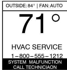
Fig. 28 - System Malfunction Screen
