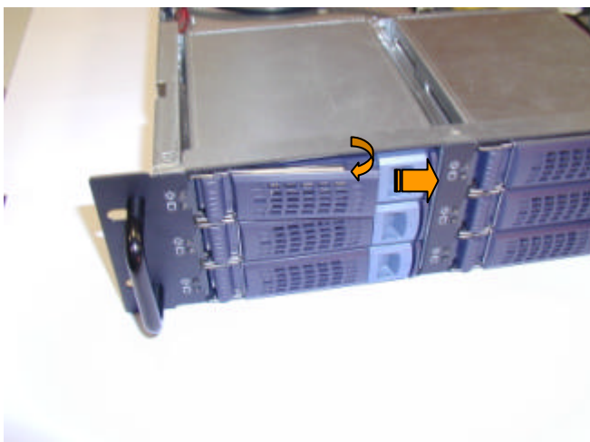
Step 6. Open the cover of HDD tray
