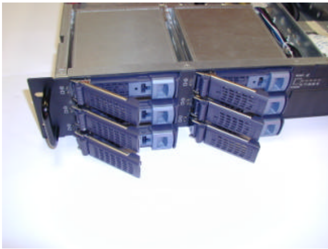
Step 8. Open all the covers of HDD trays slightly
