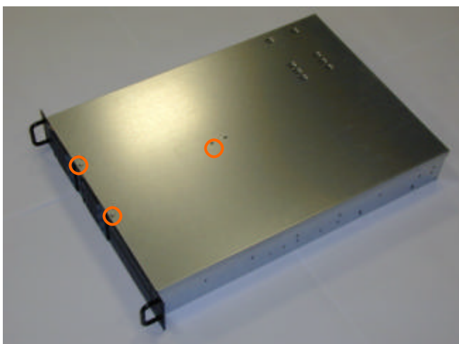
Step 36. Screw back the screws and complete the installation
