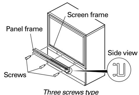
2. Insert the protective screen into the lower panel frame making sure the labeled side is to be front and the label is to be at the bottom left-hand corner.
