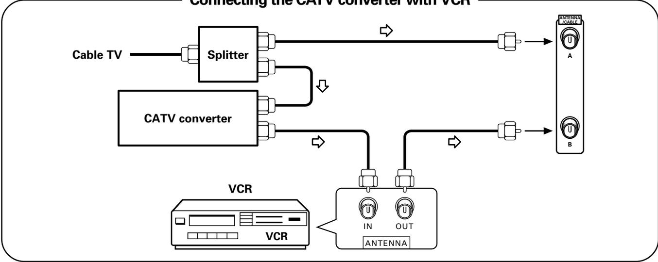
Connecting VHF/UHF antenna and CATV converter
