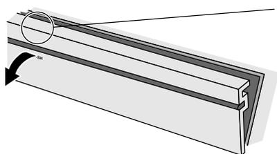
In some cases, the door may only open slightly when pushed. In such cases, open the door with your finger as shown in the figure at left.
