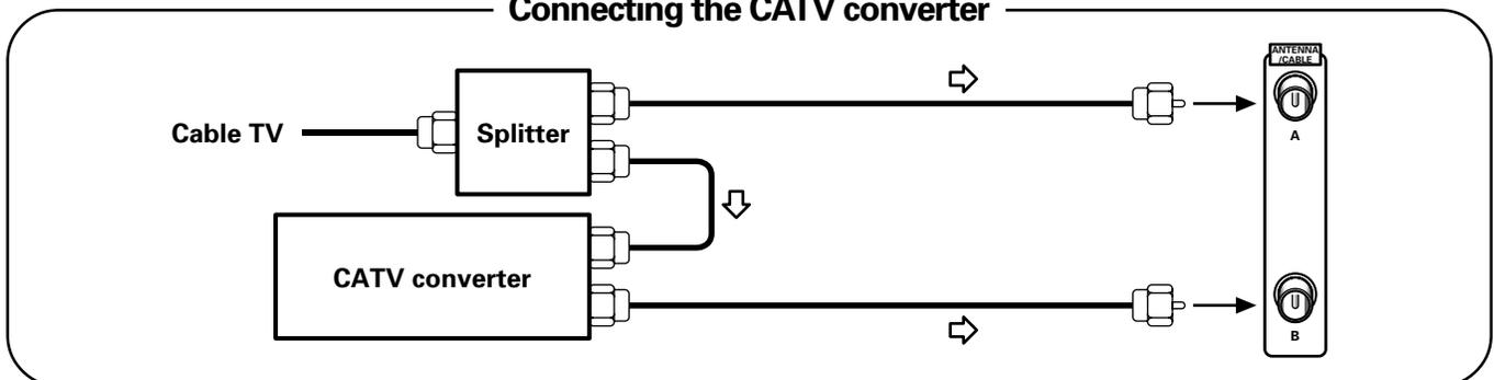
Connecting the CATV converter with VCR
