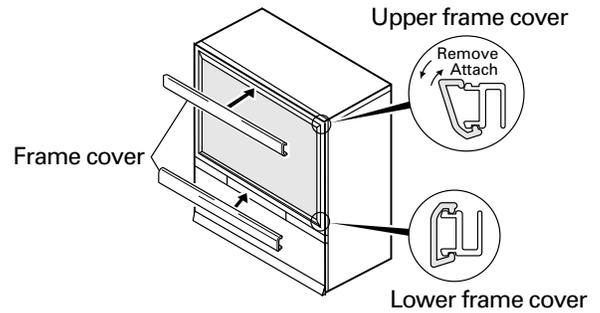
**HOW TO REMOVE THE PROTECTIVE SCREEN**
