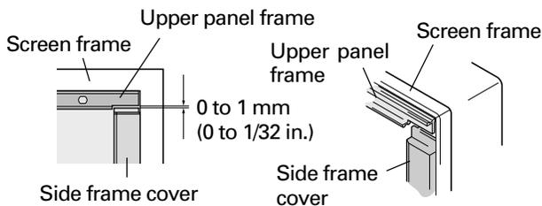
5. Attach the remaining frame covers to the upper and lower panel frames: first, insert the edge of the frame cover into the outer groove of the panel frame, then starting at one end, push the inner part of the frame cover over the inner edge of the panel frame snapping it into place.
