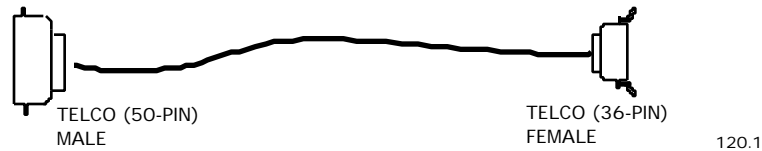
Figure 3-17. Telco 50-Pin (Male) To Telco 36-Pin (Female) Cable.
